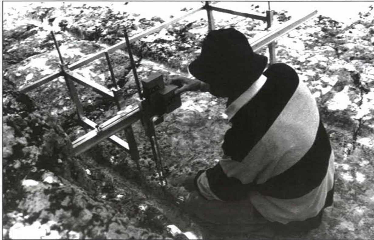
Plate 1: Instrument for measuring cart-rut profiles
